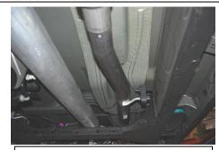
3. Install muffler assembly Item # B onto the head pipe. You may need to use a jack stand to support the muffler while installing the tailpipe. Use Item# E to clamp the muffler assembly to the head pipe. Loosely tighten
