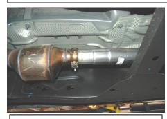
2. Install Head pipe adapter Item # G onto the factory flange. You will re use the factory clamp at this connection. Loosely tighten down the clamp. Install headpipe Item # A onto the adapter. Loosely tighten down.
