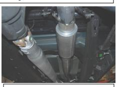
4. Install over axle pipe Item # C into the muffler outlet. Slip the hangers into the rubber grommets and keep tailpipe loose.
