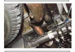
6. With proper clearance from spare tire install the exhaust tip onto the tailpipe. The system was designed to have the tip 1" below the quarter panel of the vehicle. With the tip in your desired position begin to tighten down all clamp connections from the
